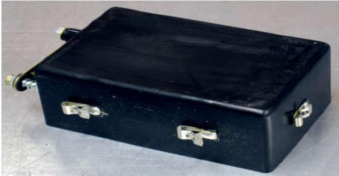
**Left clip connection is to ignition off/on switch. Middle clip goes to spark plug wire... End clip goes to the timer.**
