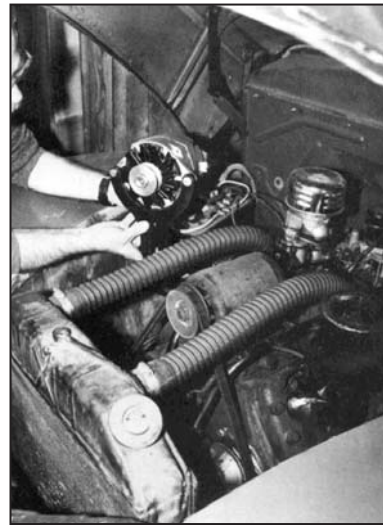
The 6-Volt Alternator ready for installation on our 1949 Ford engine.
