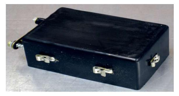
Left clip connection is to ignition off/on switch. Middle clip goes to spark plug wire... End clip goes to the timer.
