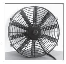
Adjustable metal brackets that mount the fan assembly to the outside framework of the radiator is the best choice for mounting the fan. Nylon ties that use the radiator core for support will damage the radiator core.
