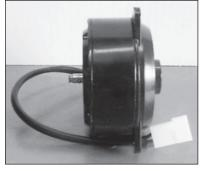
your goal in the first place. Also be aware of CFM ratings. Most do not take into consideration the radiator core thickness, and the number of fins per-inch, that make up the radiator core. A better gauge is the size of the motor, the number of blades, and the pitch of the blades.
