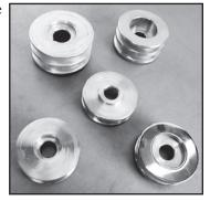
The diameter of the alternator pulley is very important. In order to insure a strong output from the alternator at idle and low rpms, it is important that the alternator pulley be at or close to (2.5") in diameter.
