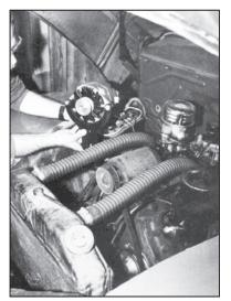
The 6-Volt Alternator ready for installation on our 1949 Ford engine.
