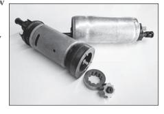
alcohol gasoline without failure. Also important is to find a fuel pump that **maintains the original fuel pump pressure**, while increasing the **volume** of fuel delivered. Too much fuel pump pressure against the needle and seat in the carburetor will result in the carburetor flooding over.
